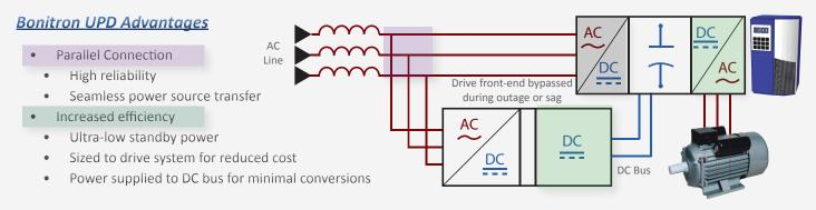
Competitors' double conversion UPS systems convert DC voltage that is stored in batteries or capacitors back to AC voltage in order to power the drive, which in turn converts it back to DC. Variable frequency drives are not recommended for use with UPS Systems, as the drive input reactance interacts negatively with UPS inverters.
