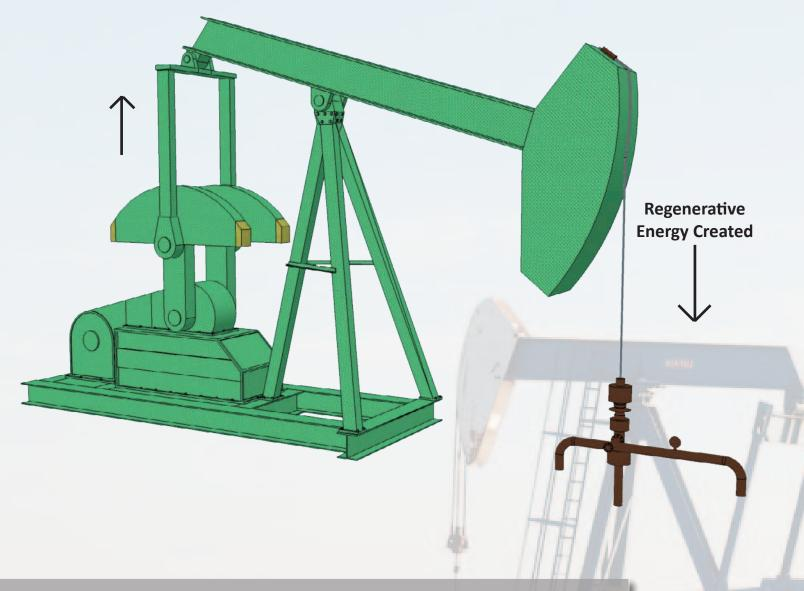
Pumpjacks are used to mechanically pump oil from the oil well when the bottom hole pressure isn't strong enough to push oil to the surface.
