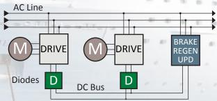
Diesel-electric propulsion systems are common in marine vessels and allow for improved maneuvering abilities and more efficient operation. A diesel-electric propulsion systems includes a diesel-driven generator, which provides electric power for propulsion, variable speed drives (VSD), and electric motors. The electric motors are able to change speed and direction rapidly, allowing for high precision movement.
