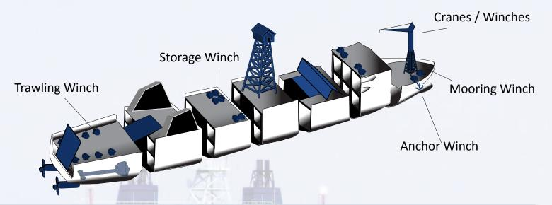
Winches are used to mechanically pull in, let out, or adjust the tension of a cable, chain, or rope. They are used in many different ways in a ship, including raising and lowering the anchor, mooring, and deploying equipment. Winches are commonly powered by a variable frequency drive and three-phase motor. When lowering a load or keeping tension on a cable, regenerative energy is created. This energy could cause overvoltage faults on the drive and bring the operation to a stop.
