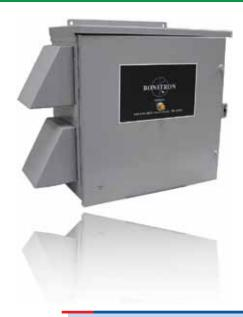
Bonitron's Model M3484 line filters are designed to be used in applications where power electronic devices experience problems from line harmonics, capacitor switching transients and DC drive notching. Typically, devices with these problems have overvoltage faults. The problems are more severe when the devices are in a standby or lightly loaded mode. For this reason, chokes alone are unable to filter the transients.
