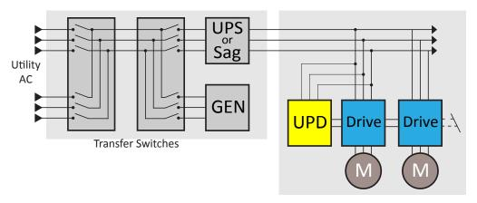
Unlike typical plant wide solutions, Bonitron designed its UPD solutions to connect directly to the DC terminals of one or multiple drives. If drive voltage sags, the Bonitron UPD immediately provides power so motor speed is not affected and the process never sees a disturbance. When properly sized, Bonitron UPD systems provide drives with full-load power until the AC line is restored or generators are online.
