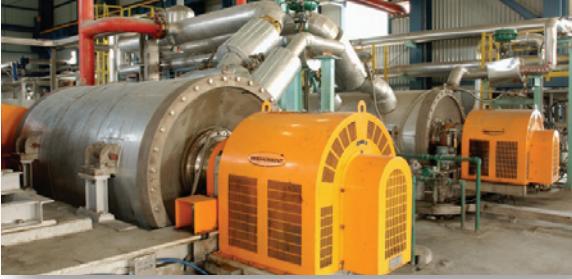
The power generated by stopping one drive can be shared to power another drive.
