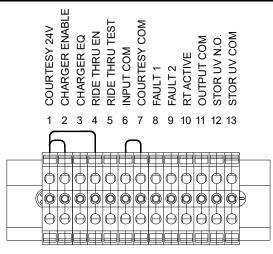
Figure 3-4: User I/O Connections with DD5 Interface Module
