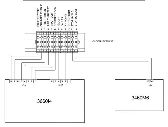
1. INVERTER AND RIDE-THRU SHOULD BE POWERED FROM THE SAME FEED TRANSFORMER. 3. ASM 3460PS WILL BE USED WHEN EQUIPPED WITH DIODE MODULE M3460D. 4. ASM 3460PS WILL PROVIDE THE DC VOLTAGE NEEDED FOR SYSTEM PRECHARGE. 2. IF LINE CHOKES ARE USED, RIDE-THRU MUST BE CONNECTED DOWNSTREAM. BRAKING RESISTOR M3460R ASM 3460PS (3) (4) STORAGE BUS RIDE-THRU DISCONNECT DRIVE DISCONNECT LINE ISOLATION TRANSFORMER M3528AC CHARGER ULTRA CAP ENERGY STORAGE BANK
