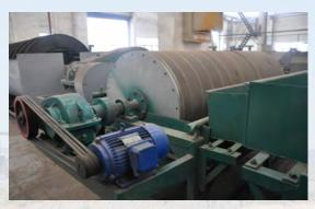
A large rotating drum that separate fine particles from coarse particles. Starting and stopping are done using VFD's.
