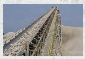
Conveyors carry limestone from the quarry to the cement plant. After the manufacturing process conveyors carry the material to the storage silos.
