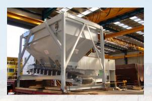
Mixers blend limestone, shale, fly ash, and bauxite. VFD's start and stop the mixing process.
