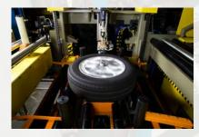
Manufacturers spin each tire up to an exact speed, precisely detect each irregularity and grind off small amounts of rubber until the tire is perfect. All this has to be done within seconds for each tire in order to keep pace with the manufacturing line.
